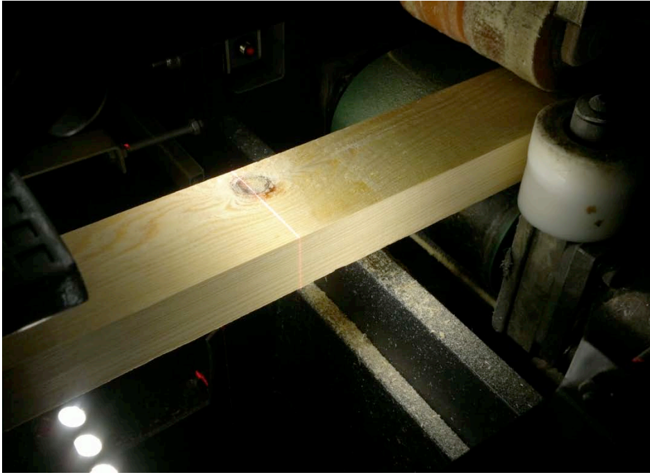
Figure 10. A piece of wood illuminated by the laser line and the white LEDs
